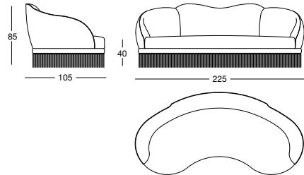
Frame in beech wood with elastic bands covered in high density polyurethane foam. Seat cushions in sterilised goose down, with insert in multi-thickness polyurethane foam.
