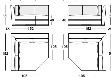
Structure in wood with elastic bands, covered in high density polyurethane foam. Backrest cushions are in sterilised goose down, with insert in medium-density polyurethane foam, and seat cushions are in triple-density polyurethane foam covered in sterilised goose down and supported with Memory Foam padding in order to maintain shape more effectively. The base of the sofa is in chromed metal in the finishes:
