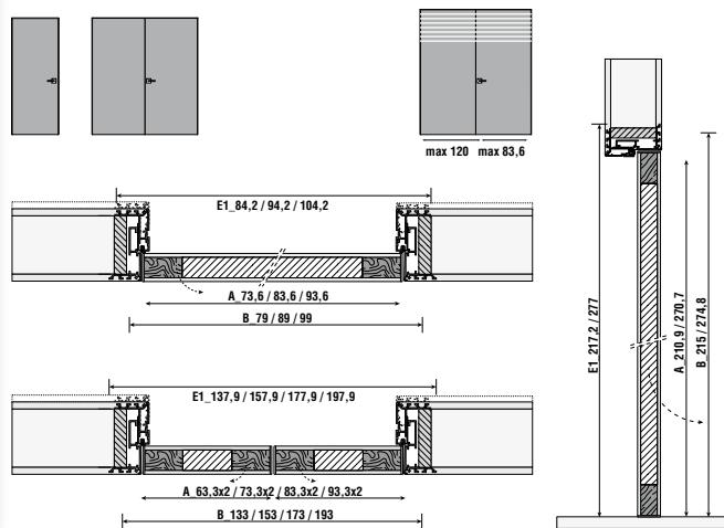
A\_Modulo / Panel - B\_Luce netta falsotelaio / Subframe measurement
