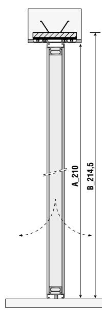
A\_Modulo / Panel - B\_Luce netta falsotelaio / Subframe measurement
