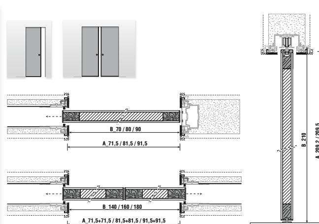
A\_Modulo / Panel - B\_Luce netta falsotelaio / Subframe measurement
