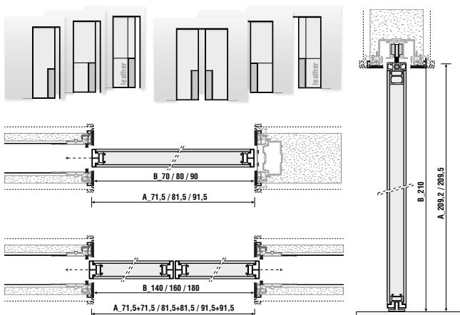
A\_Modulo / Panel - B\_Luce netta falsotelaio / Subframe measurement
